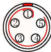
Welded surface (焊接面)
